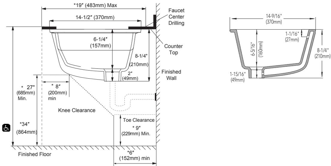
\* This sink is designed to comply with ADA ANSI A117.1 standard when installed in accordance with this measurement. Dimensions of fixtures are nominal and may vary within the range of tolerances established by ANSI standard A112.19.2. These measurements are subject to change or cancellation. No responsibility is assumed for use of superseded or voided pages.
