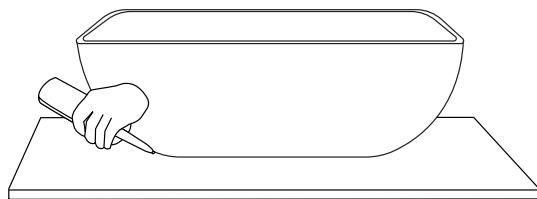
7. Remove any excess sealant with a damp cloth to complete installation.
