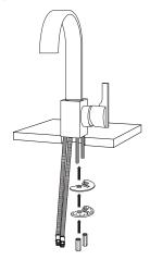
4. Attach the main supply lines to the braided water lines on the faucet. Ensure that the hot and cold lines are connected as marker. Apply plumber's tape or thread sealant to the threads before tightening. Hand tighten the connections, then finish tightening with an adjustable wrench. Be very careful not to overtighten.
