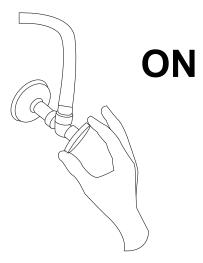
6. Proceed to sink drain installation. Once complete, turn the faucet on for approximately 60 seconds to check for any leaks. Ensure that both hot and cold water are functioning properly.
