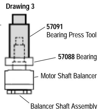
**Tool assembly is complete. Please allow 30 minutes for adhesives to cure before operating tool.**
