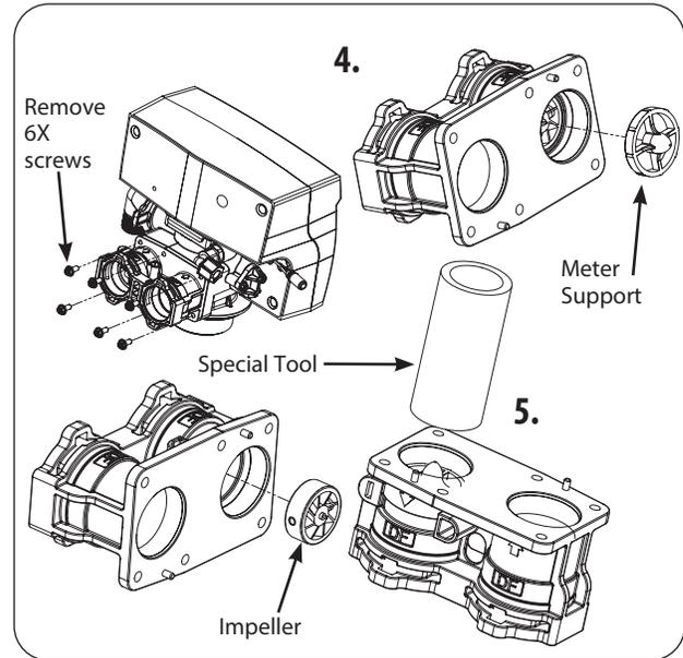
4. Remove six screws and pull out the meter support and impeller.
