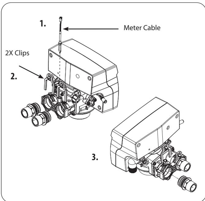
1. Disconnect the meter cable from the meter.
