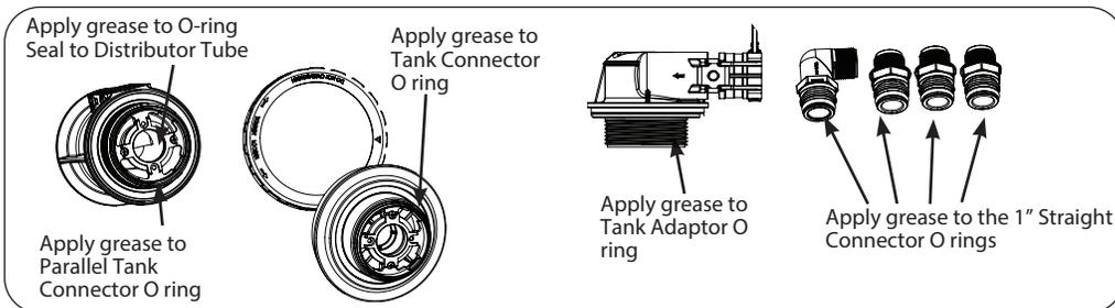
Ensure all O-ring on both tank connectors are properly disassembled and apply a good amount of grease.
