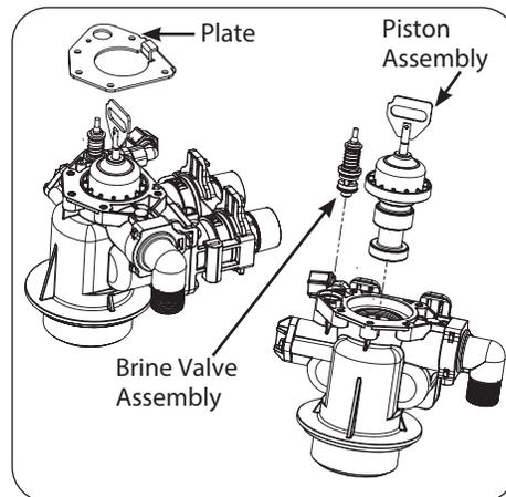
3. Remove the plate from the valve body and pull the Piston Assembly from the valve. The brine valve assembly can also be removed in this stage.
