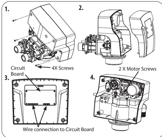
1. Remove Screws from the back of the valve and pull the cover
