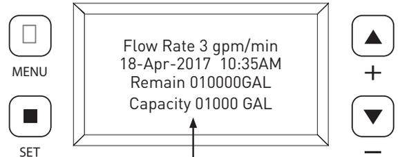
The controller will show the following on the screen: Time, Date and Gallons Remaining for Regeneration
