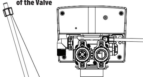
Insert Sleeve inside the Tubing
