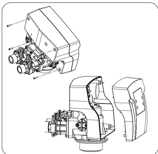
1. Remove the screws from the back of the valve and pull the front cover
