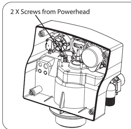
5. Remove the two screws from the powerhead as shown
