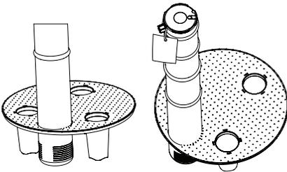
c) Drop the brine grid with brine well inside the brine tank such that the nut fitting faces the hole on the brine tank. Then press the grid evenly inside the brine tank until the brine grid legs touches the bottom of the brine tank.
