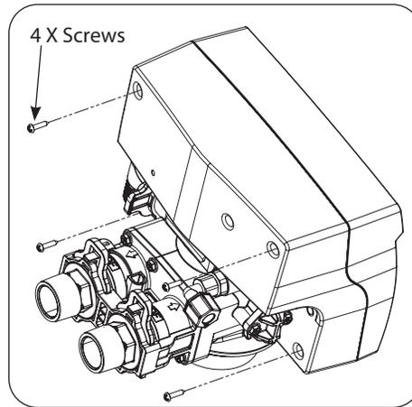
2. Remove four screws from the back of the valve cover
