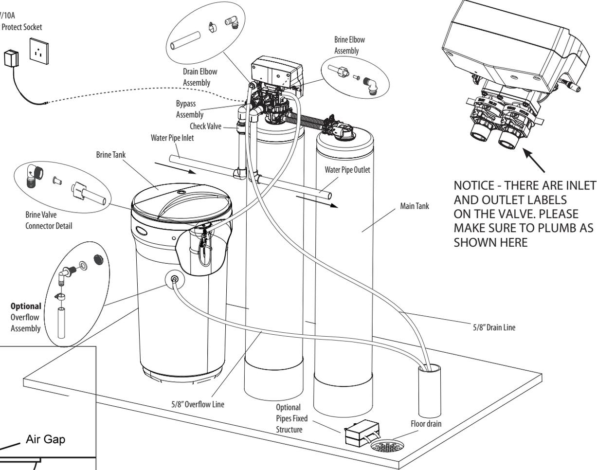
**NOTICE - THERE ARE INLET AND OUTLET LABELS ON THE VALVE. PLEASE MAKE SURE TO PLUMB AS SHOWN HERE**
