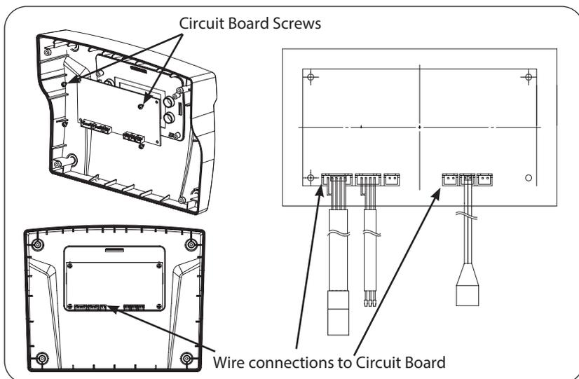
2. Remove all connections from the circuit board
