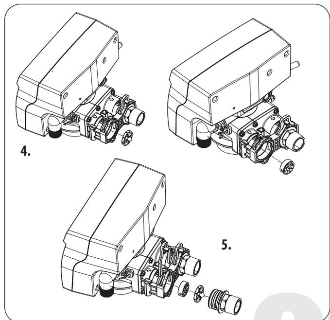
4. Remove the meter support and then the impeller out from the coupling and clean it
