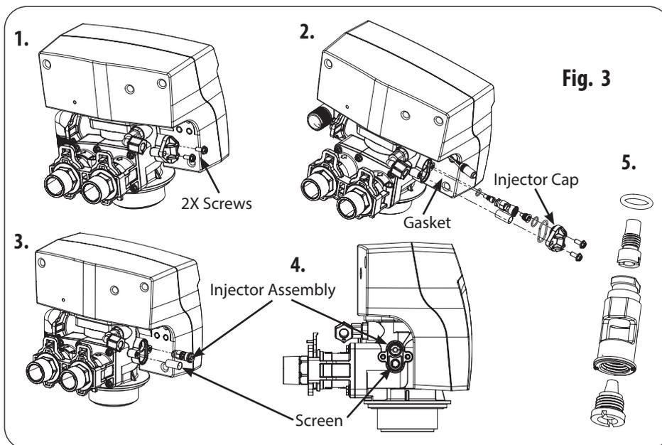
1. Remove the two screws from the injector cap
