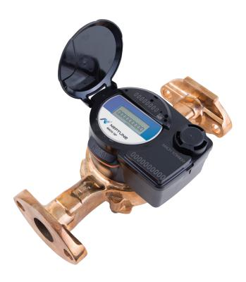
Because the Neptune® MACH 10® ultrasonic water meter has no internal parts that can wear over time, there is no opportunity for accuracy loss over the life of the meter. The MACH 10 combines solid state metrology with a corrosion-resistant, lead-free, high-copper alloy maincase, built to withstand demanding service conditions – internal water pressure, rough handling during installation, and in-line piping stresses.
