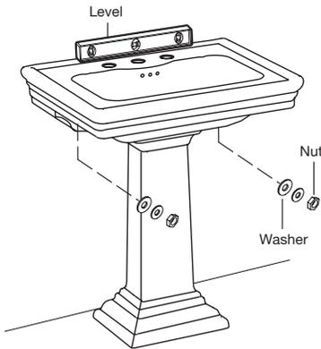
Install the nuts and washers, and tighten until snug. Connect and tighten the trap. Connect the hot and cold water supplies to the faucet.
