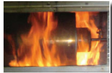
Dresser couplings were subjected to a 30 minute fire test at 1472°F (800°C), in accordance with ABS Rules and meet ISO 19921 and ISO 19922 requirements.
