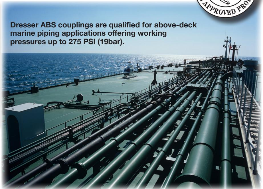
Dresser ABS couplings are qualified for above-deck marine piping applications offering working pressures up to 275 PSI (19bar).
