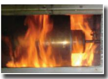
Dresser couplings were subjected to a 30 minute fire test at 1472°F (800°C), in accordance with ABS Rules and meet ISO 19921 and ISO 19922 requirements.
