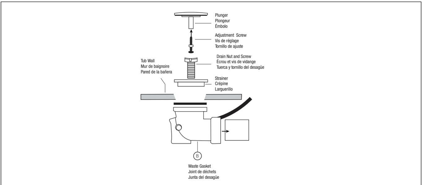
4. Making sure that waste elbow (B) and gasket are centered, place a bead of silicone sealant around strainer, and tighten drain nut and screw onto waste elbow (B).
