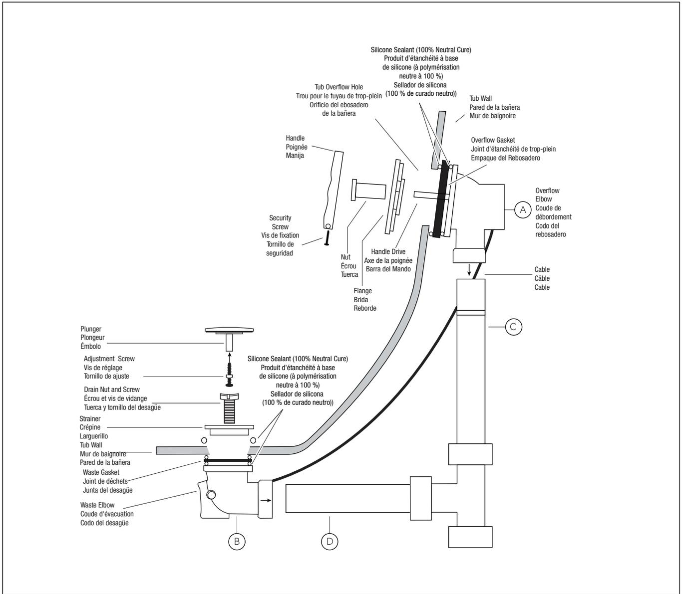
1. For ABS and PVC pipe installation apply solvent cement to outside of pipes (C&D) and inside of hub on overflow elbow (A) and waste elbow (B) and push them onto pipes as shown. Then proceed to install trim set.
