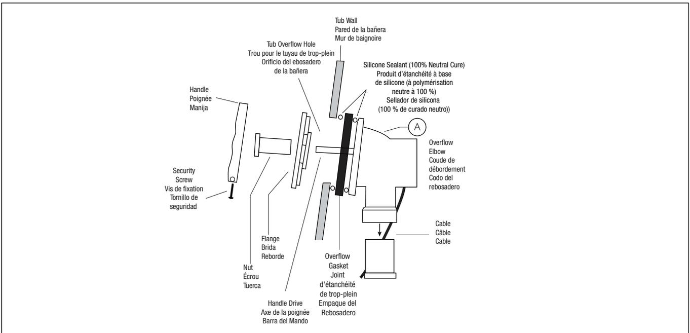
2. Put overflow washer over overflow elbow (A). Place flange over gasket and secure with nut.
