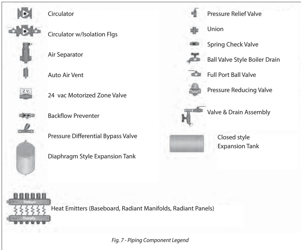
Fig. 7 - Piping Component Legend
