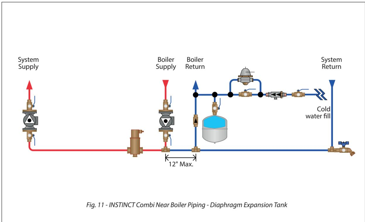
Fig. 11 - INSTINCT Combi Near Boiler Piping - Diaphragm Expansion Tank
