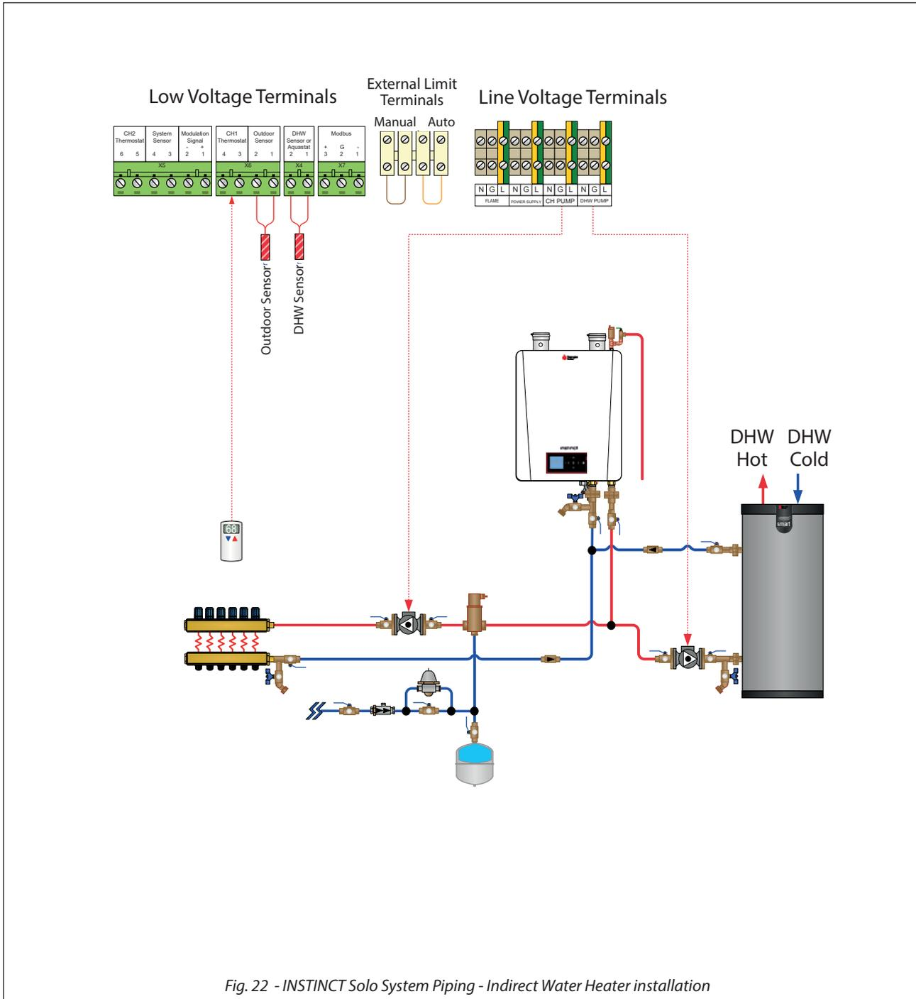
Fig. 22 - INSTINCT Solo System Piping - Indirect Water Heater installation
