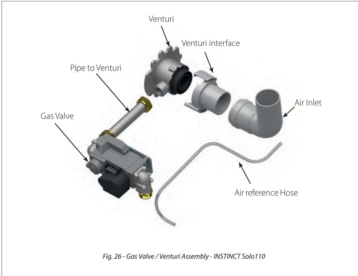
Fig. 26 - Gas Valve / Venturi Assembly - INSTINCT Solo110
