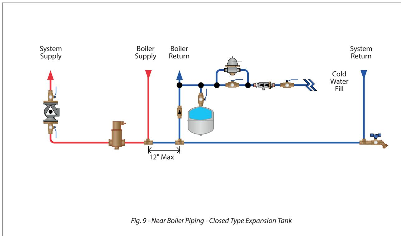
Fig. 9 - Near Boiler Piping - Closed Type Expansion Tank
