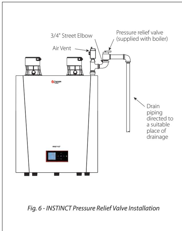
Fig. 6 - INSTINCT Pressure Relief Valve Installation
