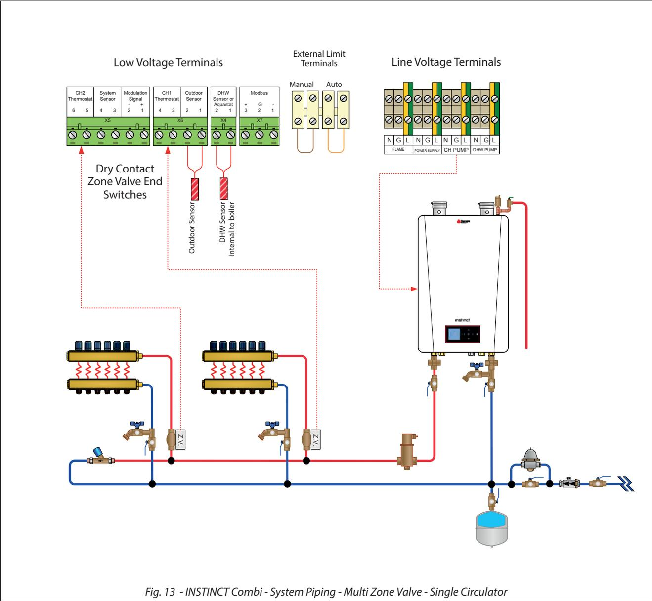
Fig. 13 - INSTINCT Combi - System Piping - Multi Zone Valve - Single Circulator
