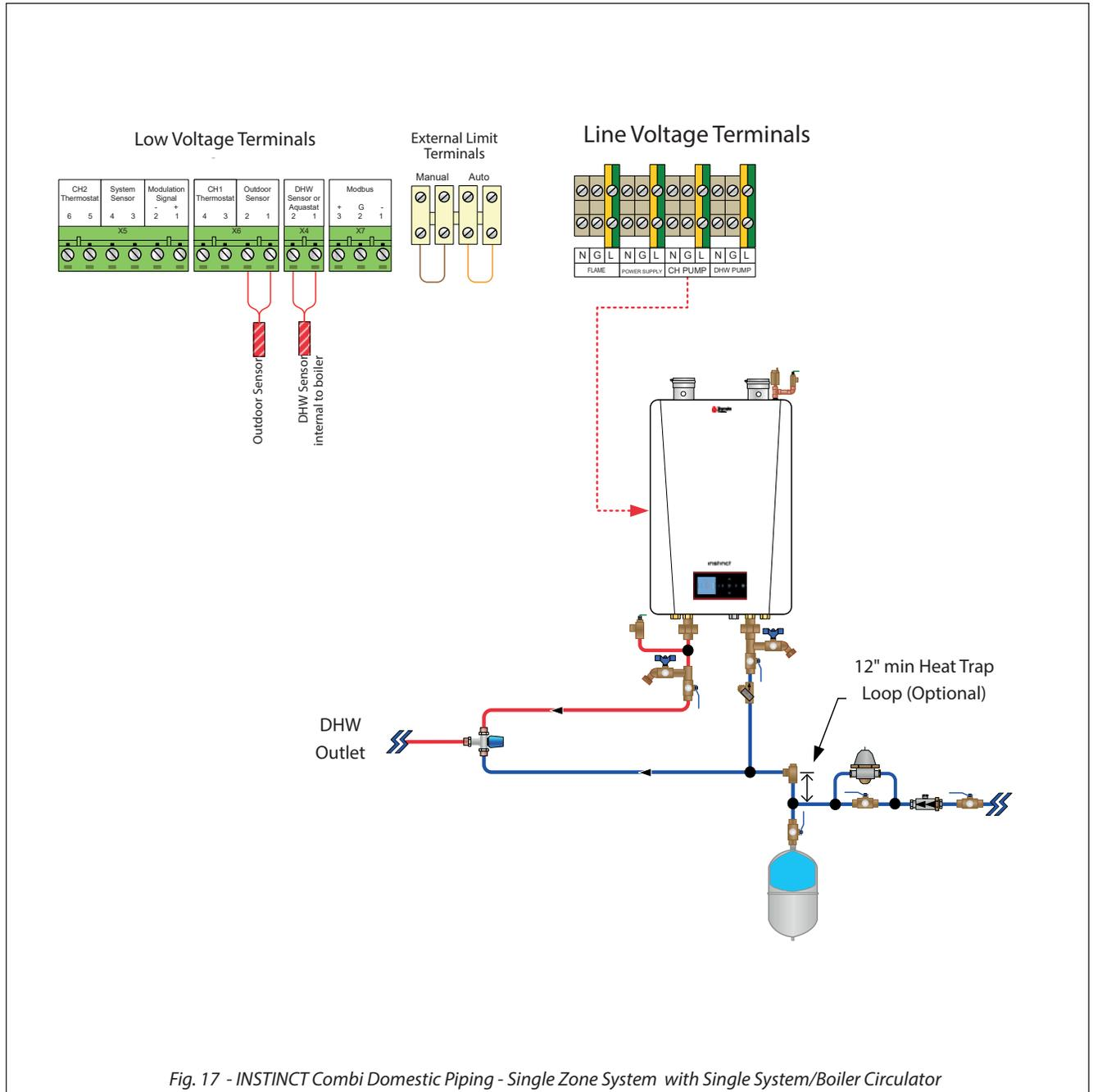
Fig. 17 - INSTINCT Combi Domestic Piping - Single Zone System with Single System/Boiler Circulator
