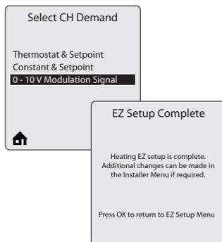
**0 - 10V Modulation Signal** - This option allows the INSTINCT firing rate to be controlled by an external control system.
