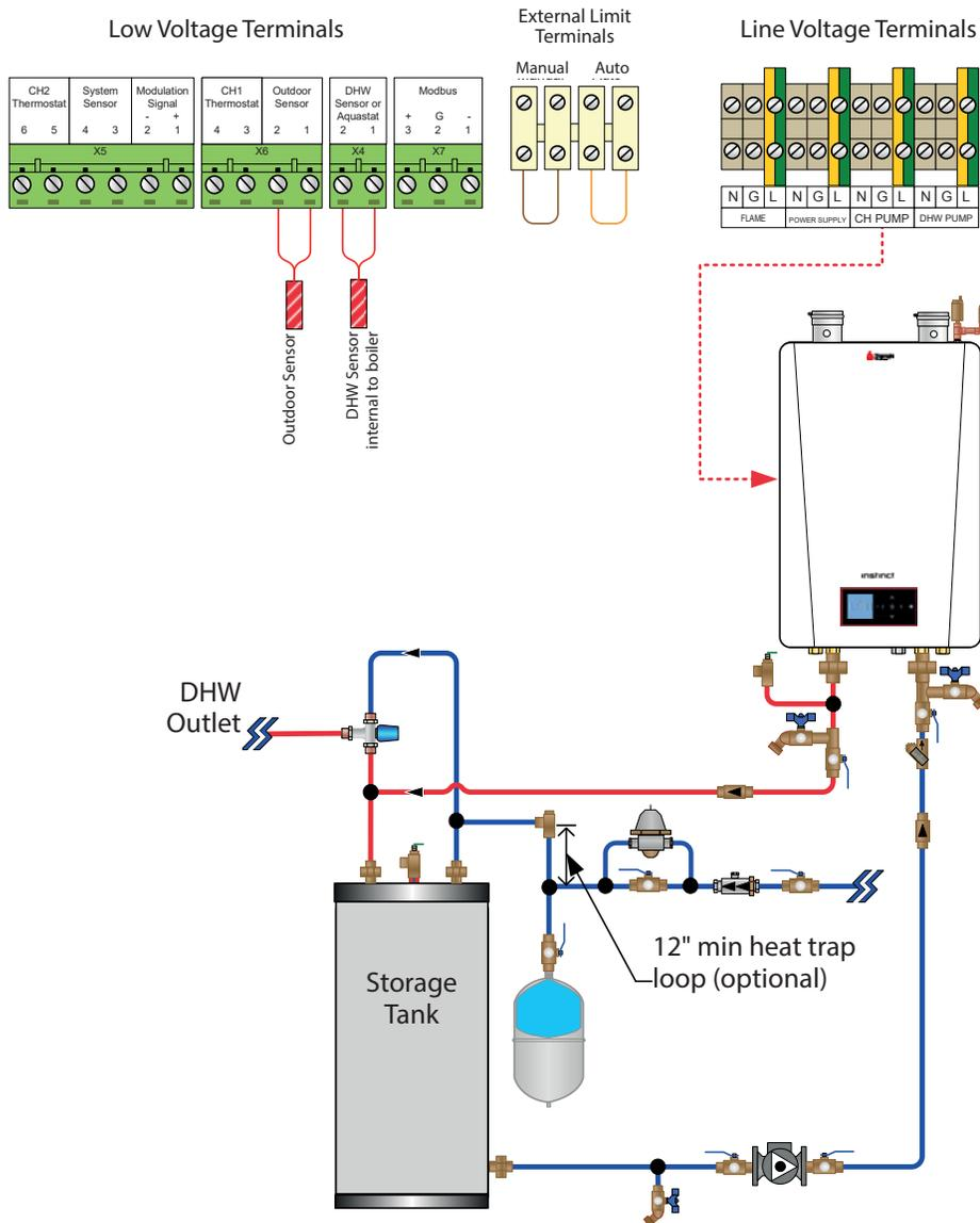
Fig. 18 - INSTINCT Combi Domestic Piping - Storage tank installation
