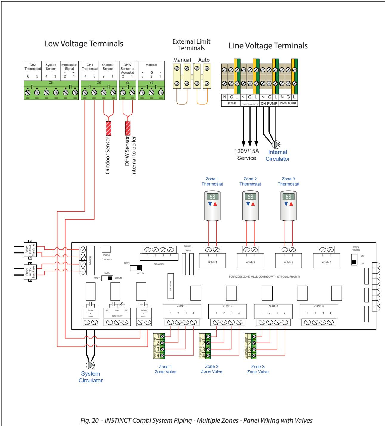
Fig. 20 - INSTINCT Combi System Piping - Multiple Zones - Panel Wiring with Valves
