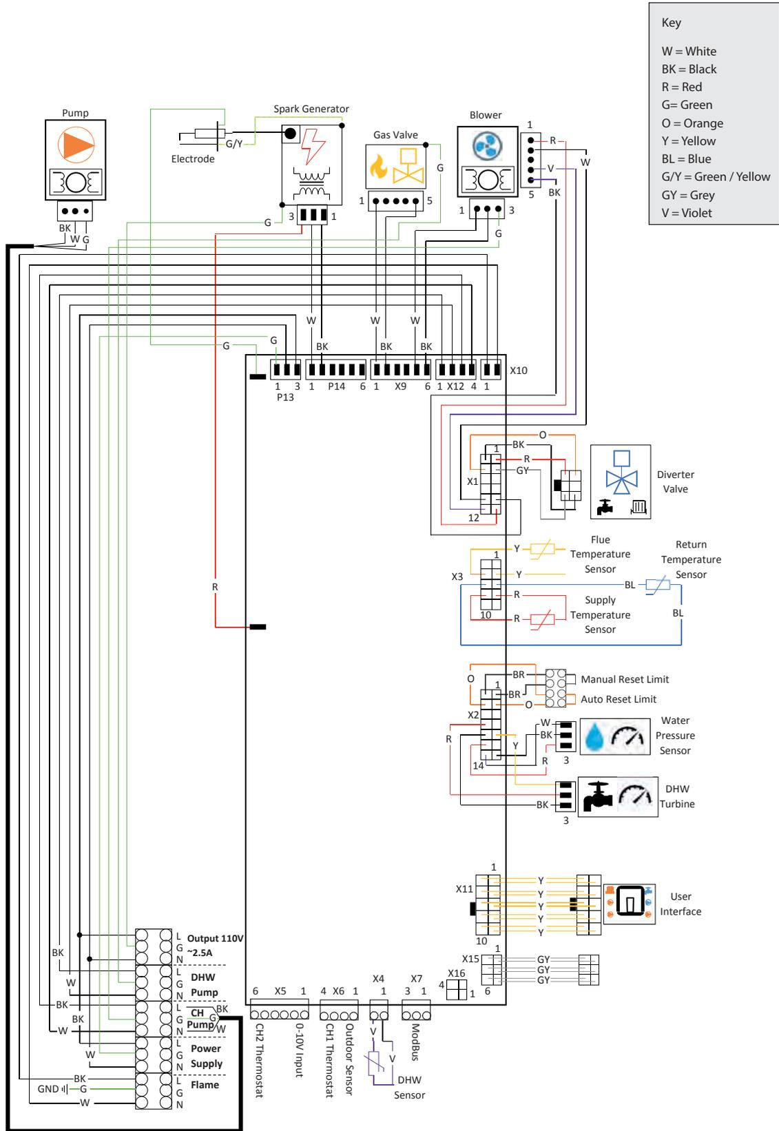
Fig. 32 - INSTINCT Combi Boiler Factory Wiring
