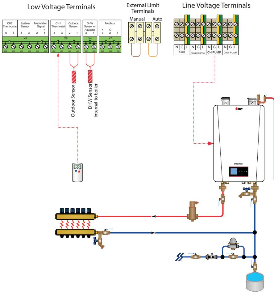
Fig. 14 - INSTINCT Combi - System Piping - Single Zone with Single Circulator
