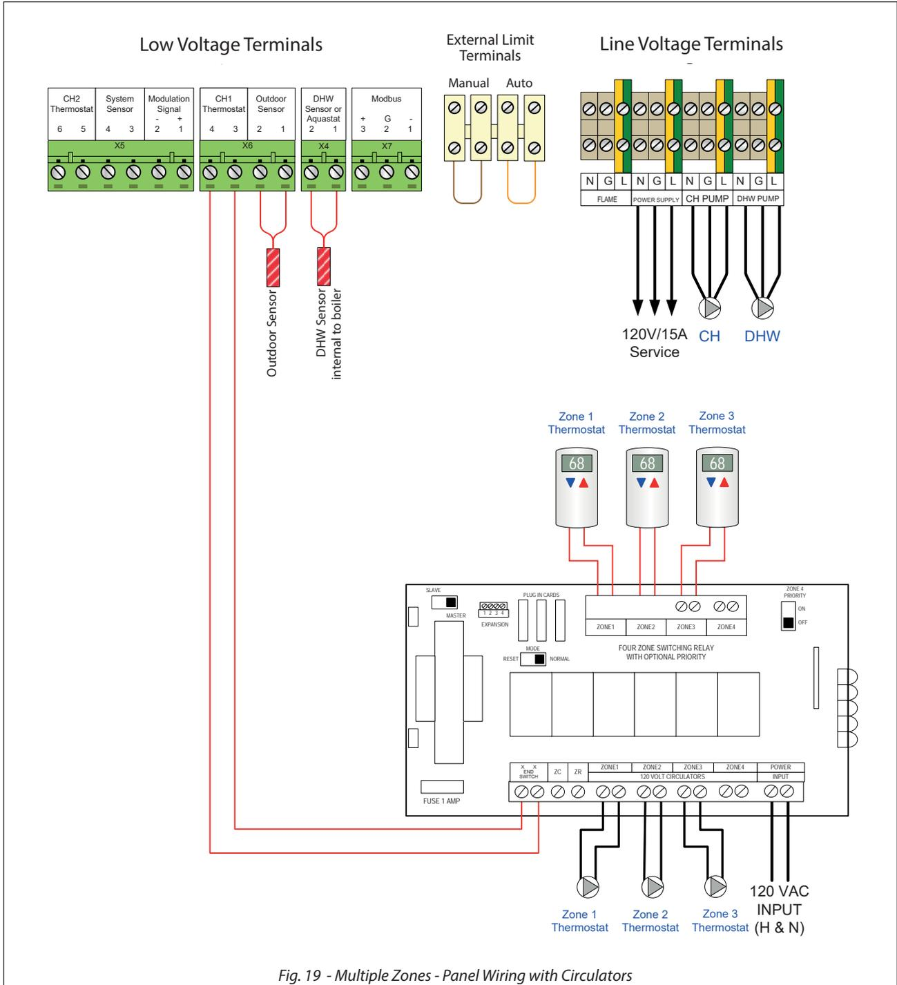
Fig. 19 - Multiple Zones - Panel Wiring with Circulators
