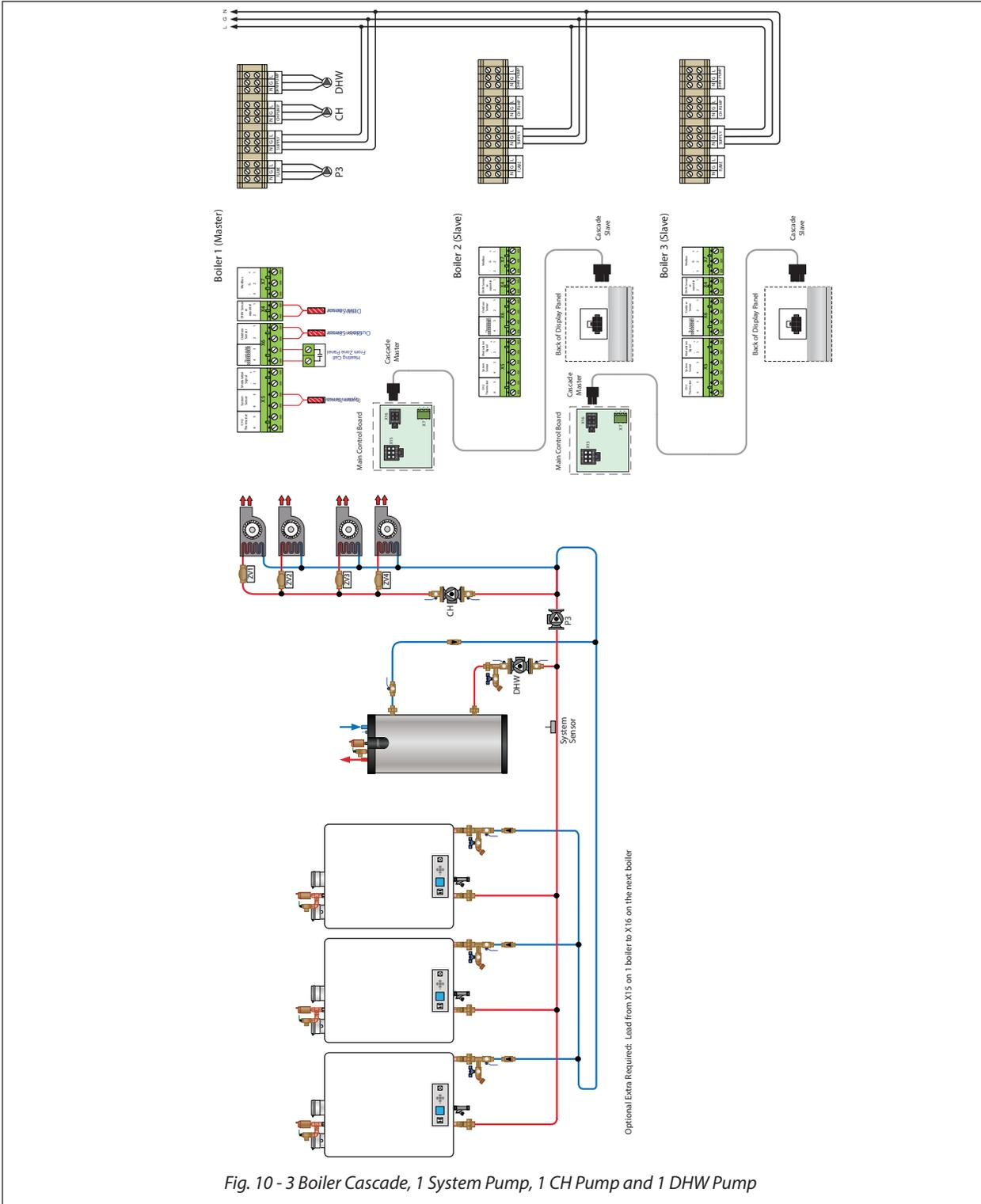
Fig. 10 - 3 Boiler Cascade, 1 System Pump, 1 CH Pump and 1 DHW Pump
