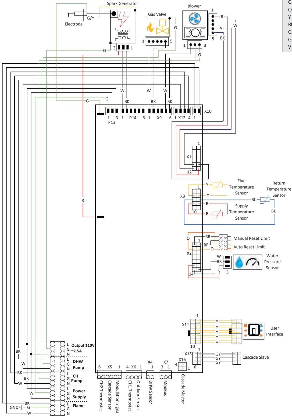
Fig. 31 - INSTINCT Solo Boiler Factory Wiring
