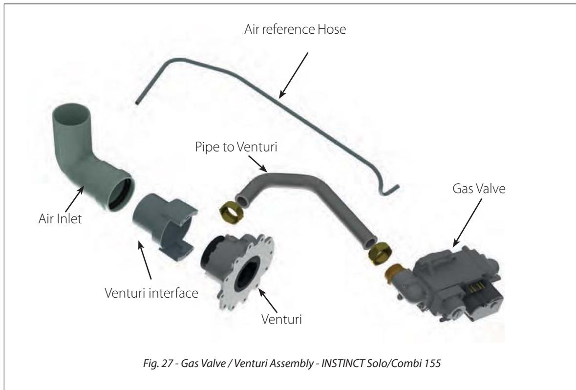
Fig. 27 - Gas Valve / Venturi Assembly - INSTINCT Solo/Combi 155
