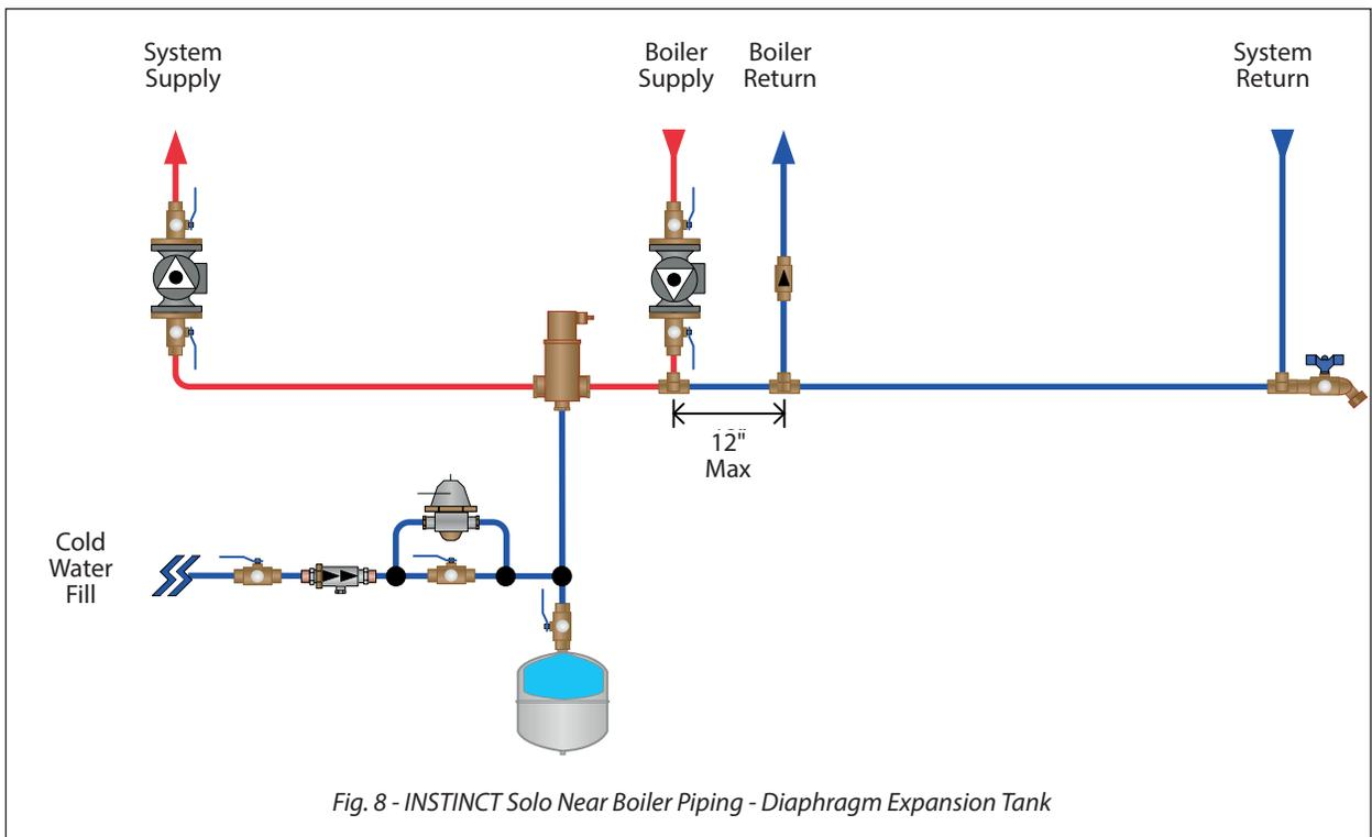
Fig. 8 - INSTINCT Solo Near Boiler Piping - Diaphragm Expansion Tank
