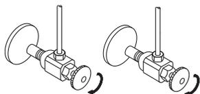
2. Remove the quick connector from the free end of the supply hose by unscrewing in a counter-clockwise direction.
