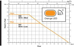
In constant pressure mode (ZV), the circulator maintains a constant pressure differential ( $\Delta p$ -c) in the system as heating load increases or decreases. Selections options are Medium or High.
