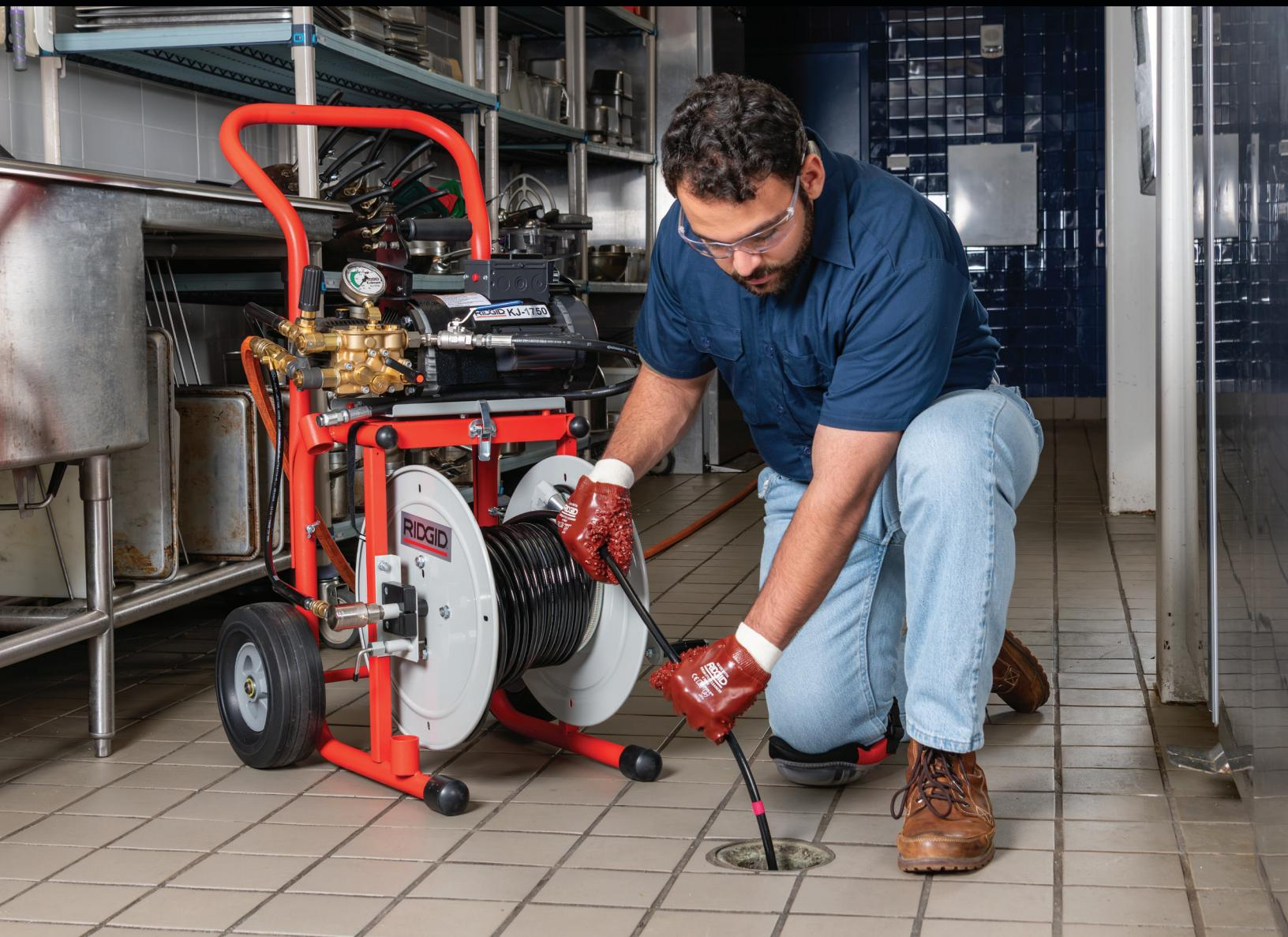
The RIDGID® KJ-1750 is a powerful electric jetter built for mid-size jobs that demand performance and reliability. Designed to tackle 1 1/4" to 4" lines, it uses high-pressure water to cut through grease, sludge, and soap buildup. As the hose retracts, it thoroughly scours the pipe interior—removing debris and restoring optimal flow.
