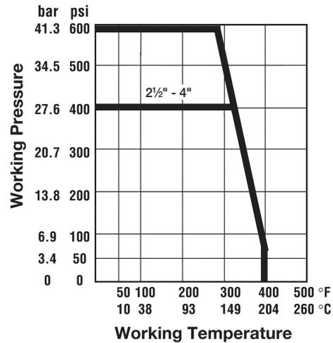
\*See application note on reverse side for solder end valves with regards to pressure/temperature rating.
