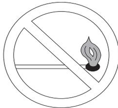
**Fig. 5 – Do Not Light Burner with Match**
