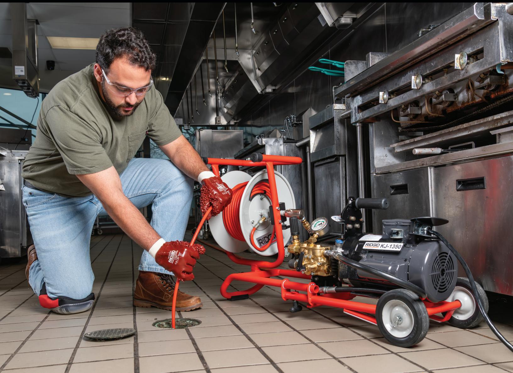
The RIDGID® KJ-1350 delivers professional-grade quality and dependable performance in a compact, electric-powered design. This jetter propels a highly flexible hose through 1 1/4" to 4" lines—breaking up grease, sludge, and soap buildup. As the hose is pulled back, it power-scrubs the pipe walls, flushing debris away and restoring full, free-flowing capacity.
