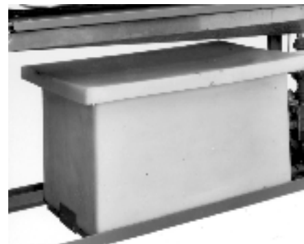
A 60 gallon covered storage tank is built into the Roto Bonder.
