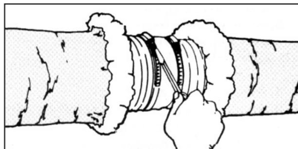
3. Pull jacket and insulation back over cores. Tape jackets together with at least 2 wraps of duct tape.
