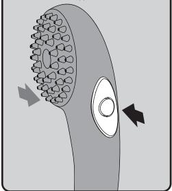
Connect remaining end of Hose to inlet of Hand Shower. Hand tighten. If there are leaks at the hose connections, look into using thicker washers to ensure a
