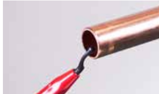
3. Use a pencil type deburrer on internal edges
