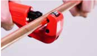
1. Cut the tube to length
