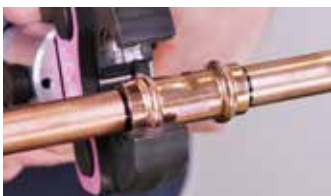
1. Align jaws square on the fitting
