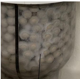
Figure 5: Salt precipitate deposited on neutralization media from Aluminum heat exchangers
