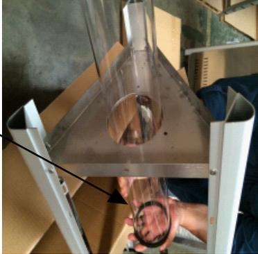
After the Glass Tube (G) is installed, be sure to wipe off all fingerprints with a clean, dry cloth.
