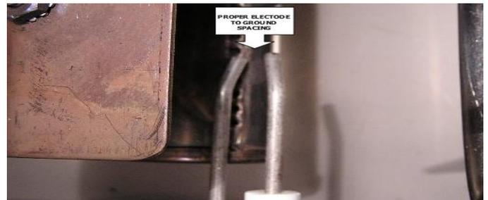
**NOTE GAP ON ELECTRODE AND GROUND WIRE SHOULD BE APPROXIMATELY 1/4"**
