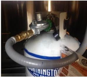
L.P. cylinder is connected to grill via a hand wheel. When full, cylinder weighs nearly 42 pounds to handle with care. Place cylinder in retaining ring and tighten screw on ring to secure tank. Place LP Regulator hand wheel in LP tank outlet, tighten hand wheel.
