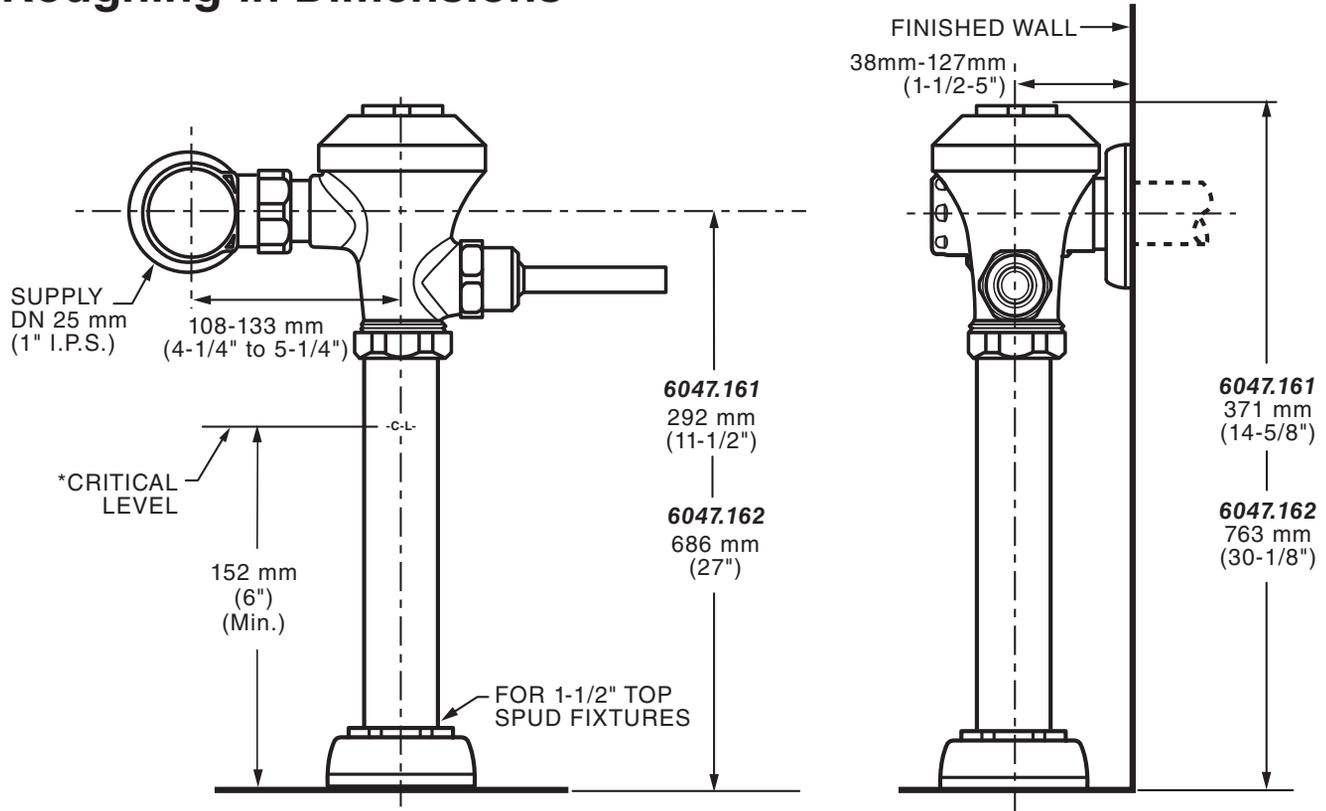
\*Note: The Critical Line (-C-L-) on Vacuum Breaker must typically be a minimum of 6" (152 mm) above fixture. Consult Codes for details.
