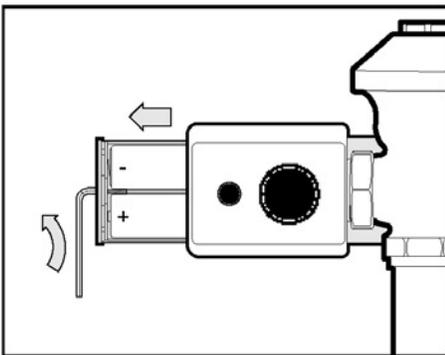
**STEP A** Use battery compartment wrench to remove battery compartment tray.
