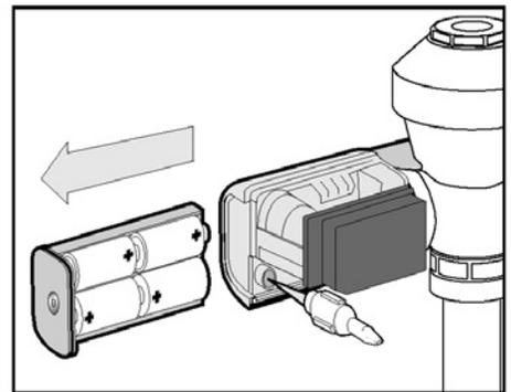
**STEP C** Sensor Adjustor Tool comes in a built-in storage pocket. Replace after use.
