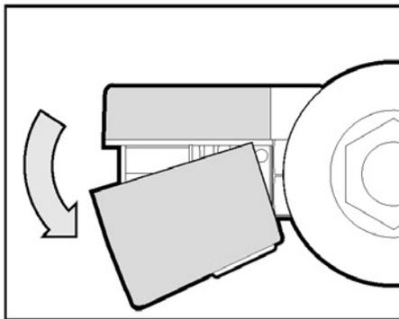
**STEP B** Pull cover off by rotating battery side forward and out.
