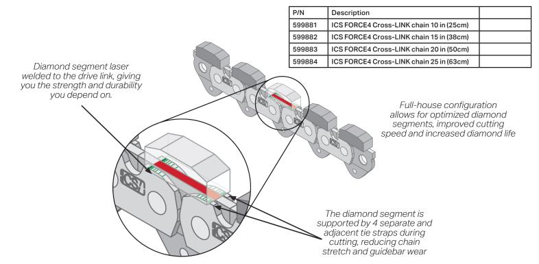
Drive Links, Tie Straps and Segments work in concert to prevent reverse articulation and increase stability in the cut, providing a smoother cutting experience with less operator effort
