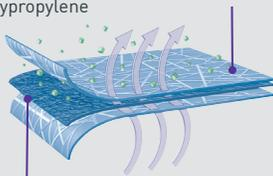
**Middle Layers** – Intricate web of microfibers that filter out many water-based liquids and dry particulates
