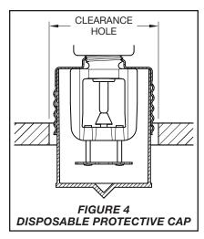
Verify that the Deflector moves up and down freely. If the Sprinkler is damaged and the Deflector does not move up and down freely, replace the entire Sprinkler. Do not attempt to modify or repair a damaged sprinkler.
