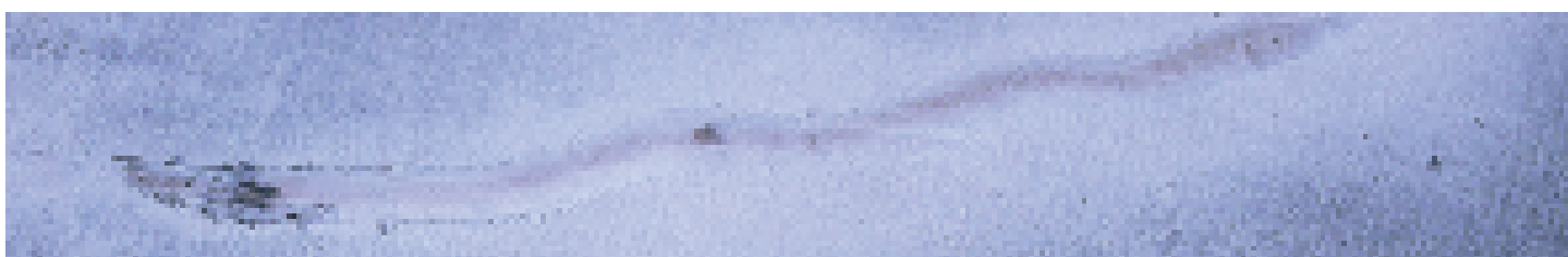
Appearance of finished crack after capping material has been ground off.
