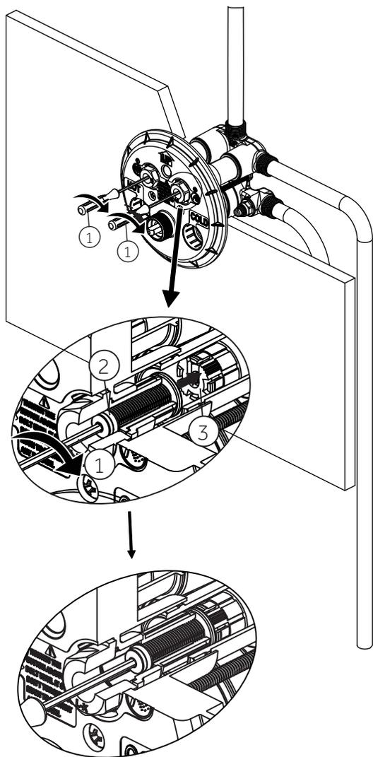
4. Loosen the stop plugs (1) with wrench and place the stop valves (1) onto the holes in the bottom of the backplate.
