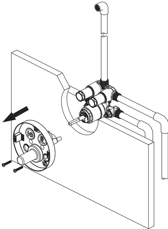
2. Secure backplate (2) to the valve body (3) with the screws (1) using Allen wrench provided.
