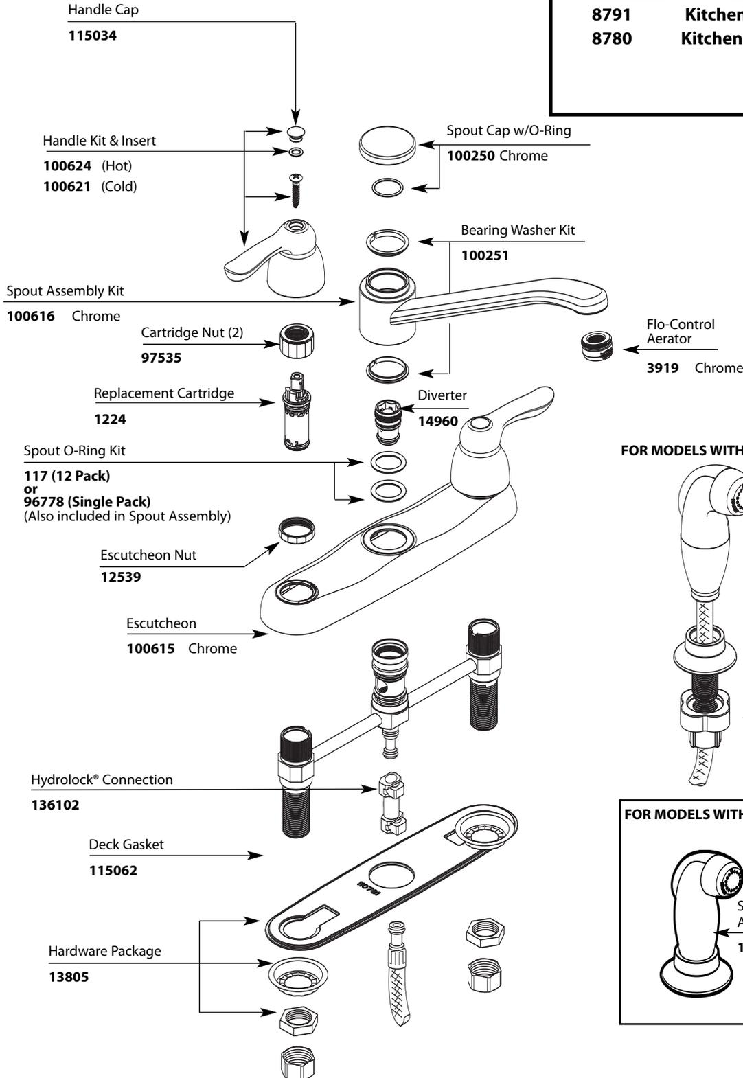
**FOR MODELS WITH HYDROLOCK<sup>®</sup> CONNECTION**
