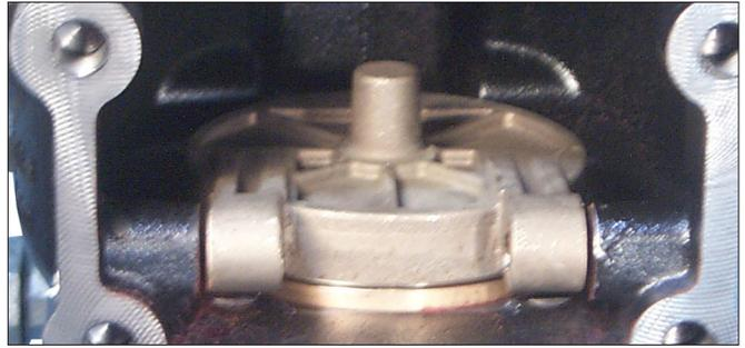
5. Place the new clapper assembly onto the valve body seat ring. Verify that the holes in the clapper arms align with the holes in the valve body.
