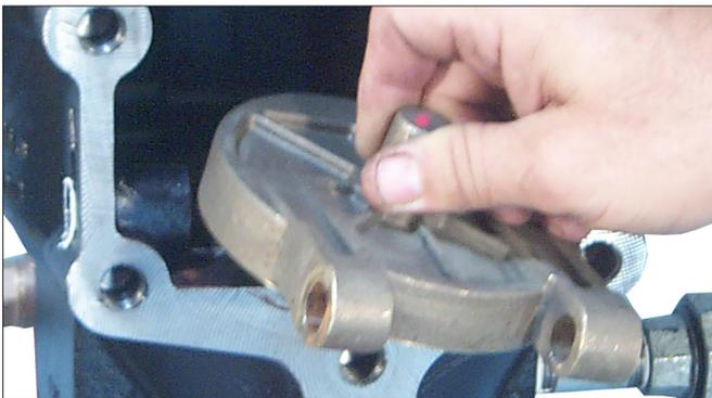
4. Remove the clapper assembly from the valve body seat ring. Clean out any holes that are plugged in the valve body seat ring. **DO NOT USE SOLVENTS OR ABRASIVES.**
