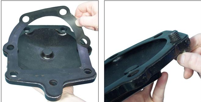
2. Align the holes of the cover plate gasket with the holes in the cover plate.
