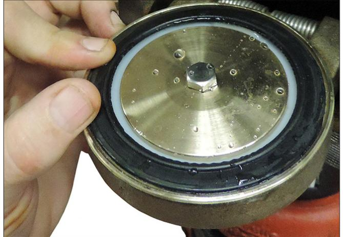
6. Rotate the clapper out of the valve body. Inspect the clapper seal and seal retaining ring. Wipe away any contaminants, dirt, and mineral deposits. Clean out any holes that are plugged in the valve body seat ring. **DO NOT USE SOLVENTS OR ABRASIVES.**
