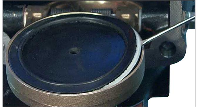
6. Pry the old clapper seal out of the clapper. For 1½ – 3-inch/ DN40 – DN80 and 8-inch/DN200 sizes, verify that the seal ring is removed with the clapper seal. Discard the old clapper seal and replace it with a new, Victaulic-supplied clapper seal assembly. Proceed to step 6a for 1½ – 3-inch/DN40 – DN80 and 8-inch/DN200 sizes or step 7 for all other sizes.
