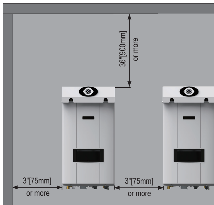
• Clearance from Wall and Ceiling
