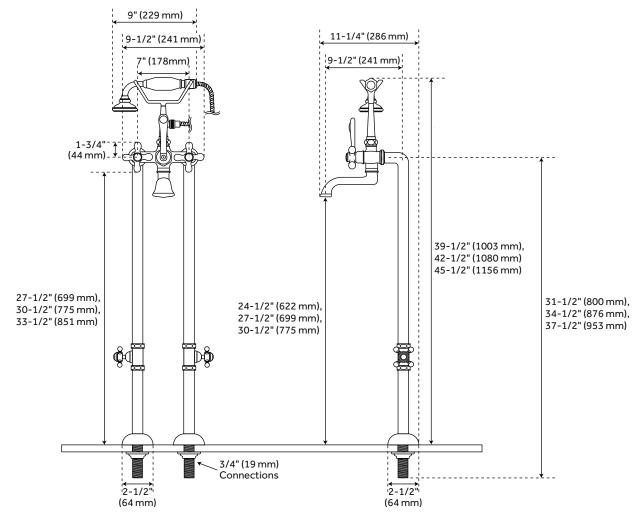
Underfloor access is required for proper installation.
