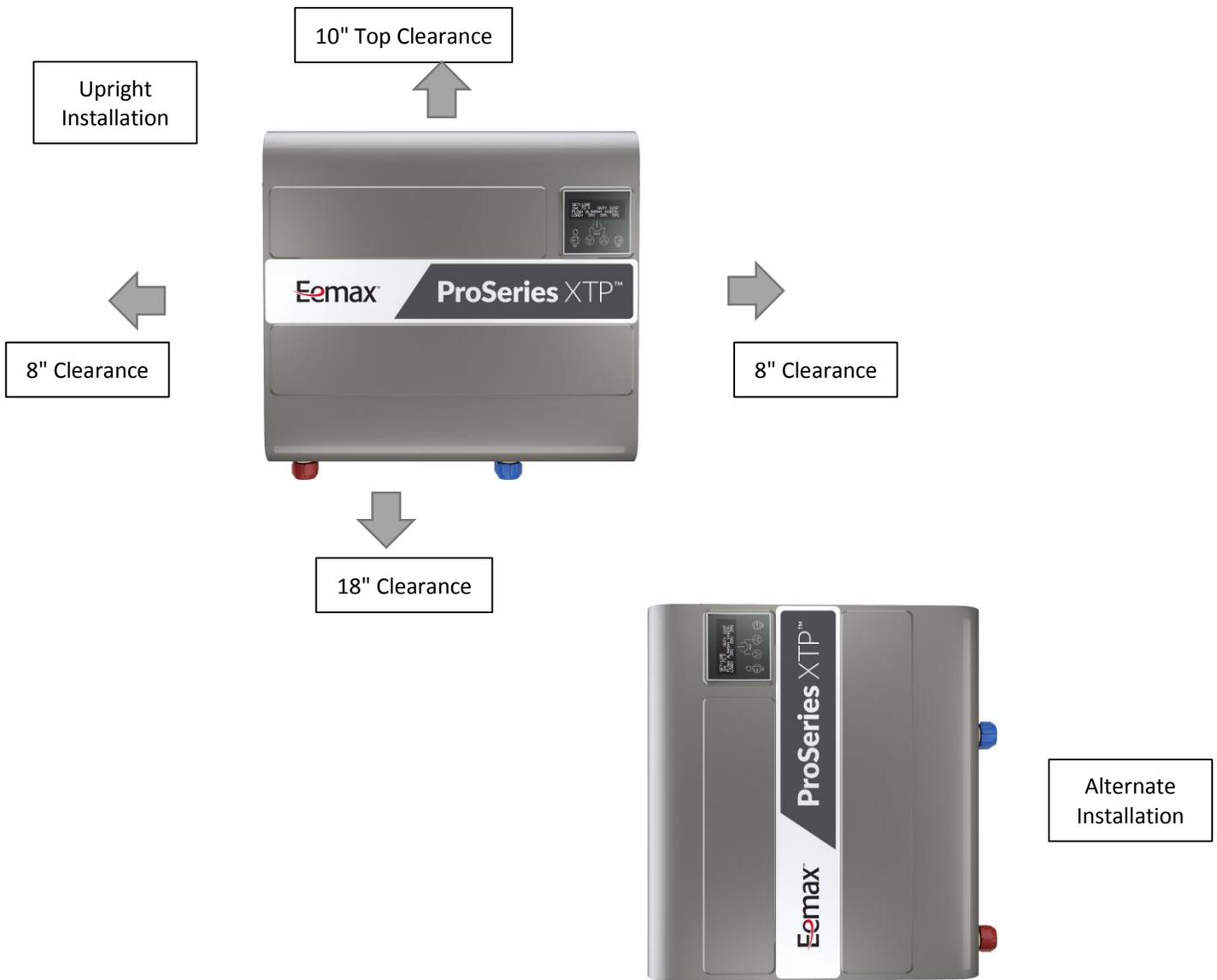
ProSeries XTP models are approved for zero clearance to combustible surfaces such as plywood.
