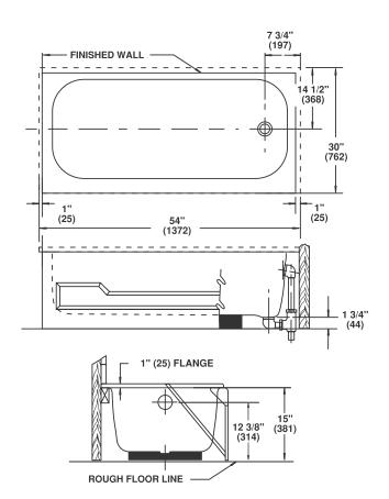
Dimensions may vary (+) or (-) 1/8". Dimensions shown in parentheses are in millimeters: 25.4 mm = 1 inch. Note: Fixture dimensions are nominal and conform with dimension and performance requirements of ASME/ANSI Standards A112.19.4M. Dimensions subject to change or cancellation without notice. Briggs is not responsible for the use of superseded or voided specification information.
