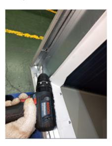
**STEP 3** - Place heat shield as shown with flanges down, and align the thru holes of the shield with the engagement holes of the coil support. Install the four screws previously removed from Step 2.
