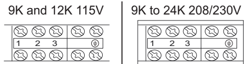
Fig. 21 — Control and Power Wiring on the Indoor Unit
