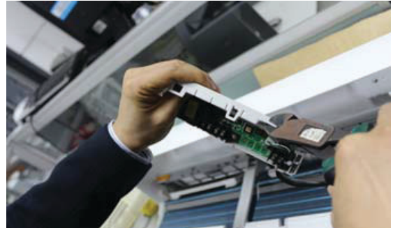
Fig. 30 — Cut a hole on the multi-function board
