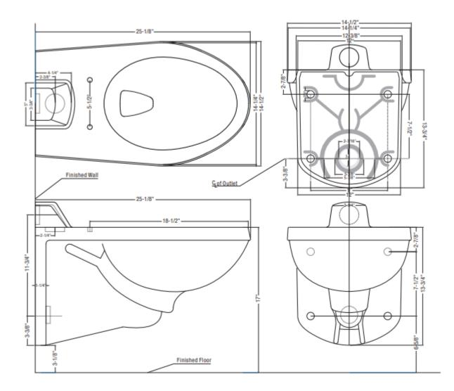
Note: All dimensions and specifications are nominal and may vary: Dimensions of 8" and greater have a tolerance of +3%. Dimensions less than 8" have a tolerance of +5%.
