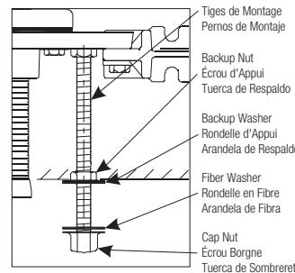
Cutaway of Mounting Hardware
