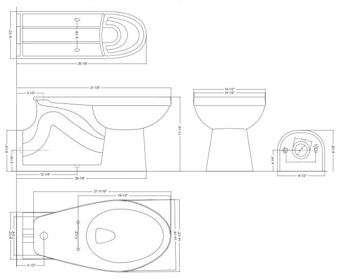
All dimensions and specifications are nominal and may vary. Dimensions of 8" and greater have a tolerances of +3%. Dimensions less than 8" have a tolerances of +5%.
