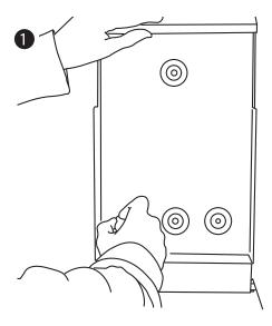
Position the dispenser against the desired spot on the wall where it will be mounted. Use a marker to mark the position of the outside three holes where the holes should be drilled. A spirit level should be used to make sure the dispenser hangs straight.
