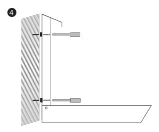
Insert the provided 1.4" inch screws through the dispenser into the provided black rubber distance holders which are placed between the wall and dispenser. Screw the dispenser into position.
