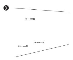
Insert the provided plastic anchors into the drilled holes.
