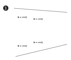
Insert the provided plastic anchors into the drilled holes.
