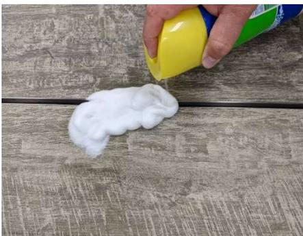
2. Using a cleaning agent as recommended above, apply an ample amount into the Drain Channel from the top side and also into the Main Channel through the Access Opening.
