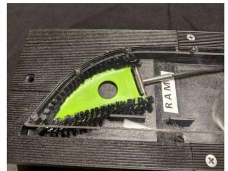
**Note: Make sure to push the D-shaped Brush to the end of the channel, moving any debris to the Drain Channel. (Tile not shown for clarity)**
