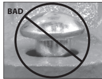
OVAL NECK OF BOLT NOT SEATED PROPERLY
