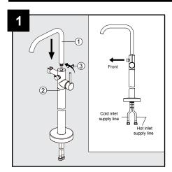
Insert the spout (1) into the faucet assembly (2). Rotate the spout (1) to align correctly with the faucet assembly (2) then tighten the set screw using hex wrench (3).
