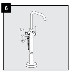
Make sure washer (1) is in hose end (2). Thread hose onto outlet (3) and tighten securely. Do not overtighten.
