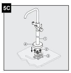
Align the faucet assembly (1) onto the rough-in body (3). Secure the faucet assembly (1) to the rough-in body (3) using bolts (2, contained in SKU# PT61000). Place the flange (4) over the standpipe and then push it to the base.
