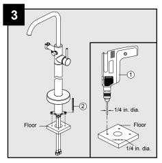
Drill a hole 2 1/4 in. diameter min. - 2 9/16 in. diameter max. in the floor with an electric drill (1). Lower the filler assembly over the hole and mark the locations for the screws with a pencil (2). Then drill four holes 1/4 in. diameter for the screws in the floor with an electric drill (1).
