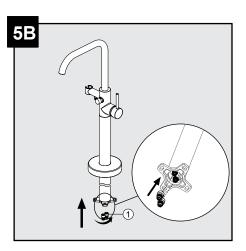
Screw the connectors (1, contained in SKU# PT61000) into faucet assembly using allen wrench .
