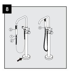
Make sure washer (1) is installed in hose end (2). Hand tighten hose onto hand shower (3). Place hand shower into holder (4). Inspect for leaks at arrows.
