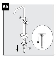
Loosen the supply hoses (1) using wrench.
