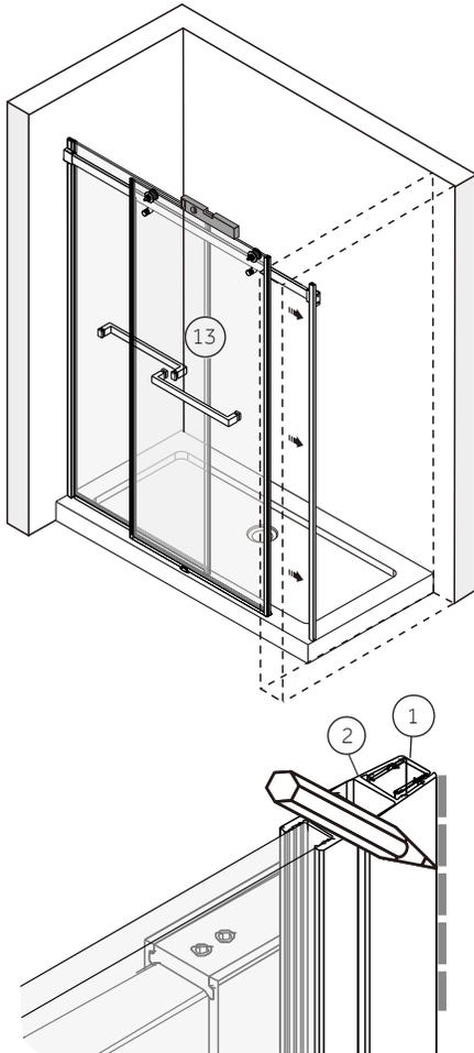
12. Note distance from wall to door guide (19), then cut threshold (16) to your noted distance less 1/2". Mark a hole for the threshold cover (15) for installation. Drill installation hole with 1/8" drill bit. Attach threshold cover (15) to tub rim with 1-1/4" screw (8).
