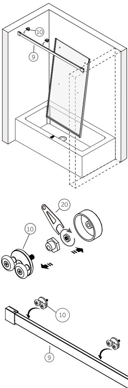
6. Insert inner door (3) onto the door guide (19) slot. Attach the inner door panel (3) to the top rail (9) with the double roller (10). Tighten the hexagonal nut with spanner (20).
