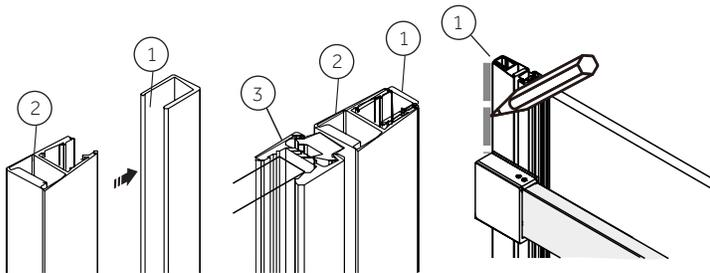
8. Install roller (11) on outer door (13), then tighten with spanner. Install threshold gasket (17) at the bottom of outer door (13). Using cutting pliers, trim the top 4-3/4" strip of the water-retaining gasket (18). Be sure to not cut the U-shaped portion of the gasket. Install water-retaining gasket (18) on outer glass (13).
