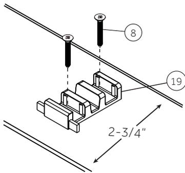
2. Disassemble the rail wall bracket kit (7) as shown. The mounting bracket kit (7) should be mounted 7/8" back from edge of door guide (19). The mounting bracket should be mounted 59-1/2" from the tub rim as shown. Drill installation hole with 1/4" drill bit. Apply a small amount of silicone sealant to the installation hole, then insert wall anchor (6). Attach rail wall bracket against the wall with 1-1/4" screw (8).
