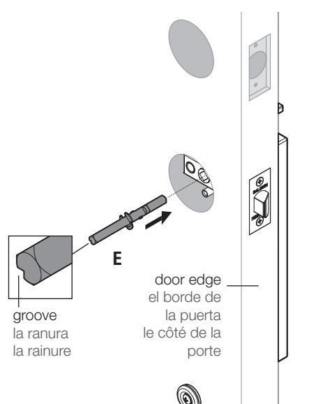
**b** Push the spindle into the hole until the notches touch the latch. If the spindle gets stuck, lift the handset to help align the holes, and push the spindle into position.
