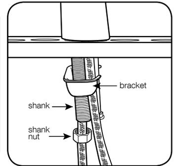
4. Below the sink, slide mounting bracket over spray hose and secure to shank with nut. Do not pinch hoses with mounting bracket. Hand tighten. Check faucet position. Secure nut with wrench.
