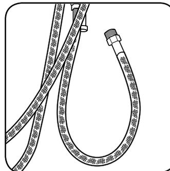
6. Make sure the spray hose is clear of supply lines and other obstructions below sink.
