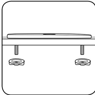
2. Below sink, secure cover plate with black mounting bolts on each post.
