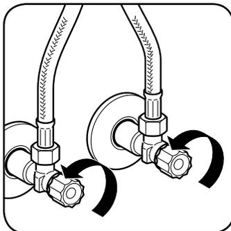
5. Before connecting supply hoses, flush lines. Attach the compression hoses to the supply stops with wrench. Do not overtighten. Hoses are color coded, red for hot and blue for cold.
