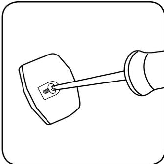
8. Using a phillips screwdriver, disassemble the weight.
