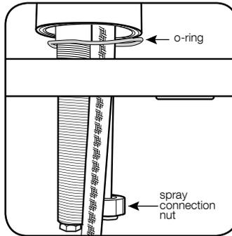
3. Position large o-ring in groove at bottom of spout. Insert faucet hoses and shank through sink hole.
