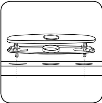
1. Install two posts into bottom of cover plate. Position cover plate and gasket over holes in the sink.
