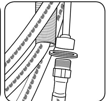
7. Insert the male end of the spray hose into the washer and copper outlet. Hand tighten and then secure with a wrench. Do not overtighten. Open the faucet and check for leaks.
