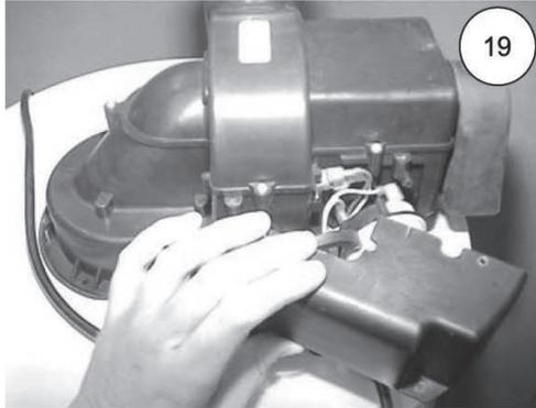
Remove three screws (Phillips Screw driver) from control access cover on blower and remove cover (see photo 19).
