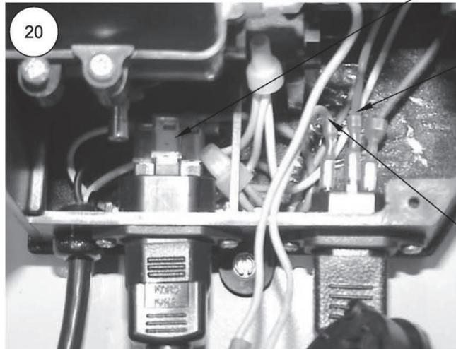
If burner does not light, observe LED flash code on gas valve and refer to troubleshooting section on page 15
